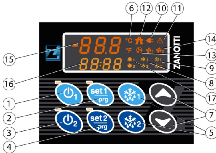
Figure 9 - Controls of main control unit (in-cab controller) - Multi temperature version
