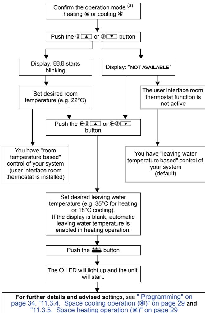
(a) The operation mode can not be selected on the hydrobox. The hydrobox follows the operation mode of the master VRV DX Indoor Unit. Refer to outdoor unit manual for further information
