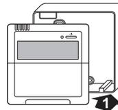
5 Remove the user interface cover from its hinge.
